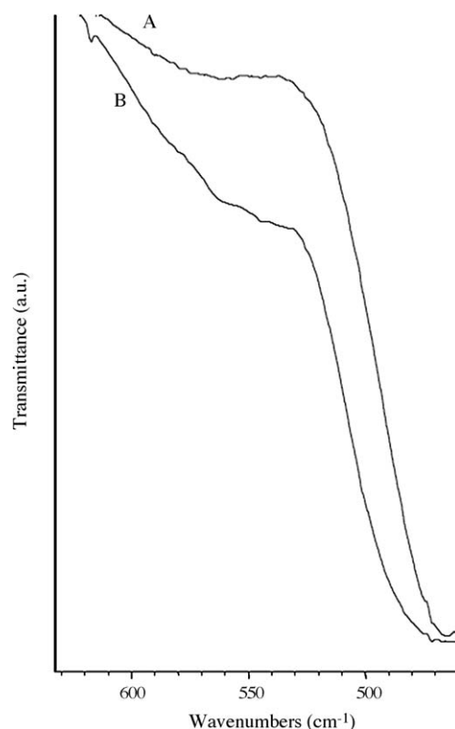
Fig. 2. FT-IR spectra of the skeletal region for SBA-15 (A) and HMFI-SBA-15 (B).
